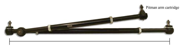
Clydesdale shown in "stock" tie rod under configuration. Photo may vary slightly from what you receive. This photo is here to show basic info. Center to center measurement should be taken like in pic above.
